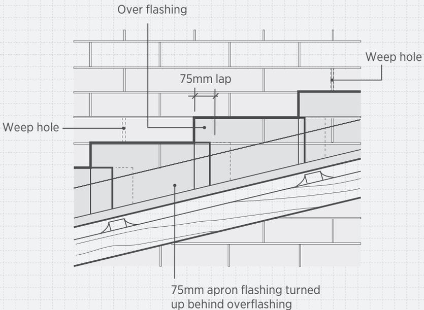
FIGURE 7.1D APRON/COVER FLASHING
