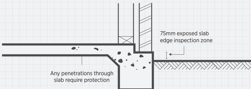
FIGURE 17.3B 75MM INSPECTION ZONE WITH METAL CAPPING
