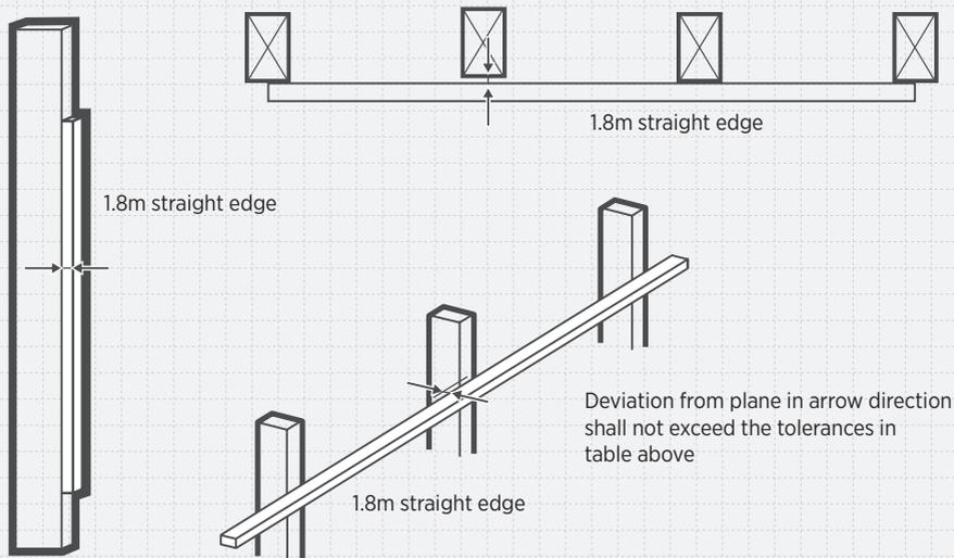
Extract from AS2589 - Gypsum lining: Application and finishings<sup>5</sup>
