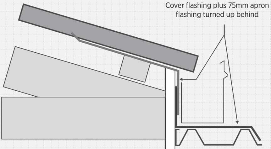
FIGURE 7.1F ANTI-CAPILLARY BREAKS
