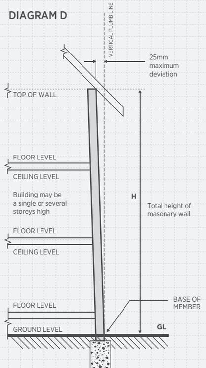
FIGURE 4.4 TOLERANCES IN MASONRY CONSTRUCTION CONTINUED.
